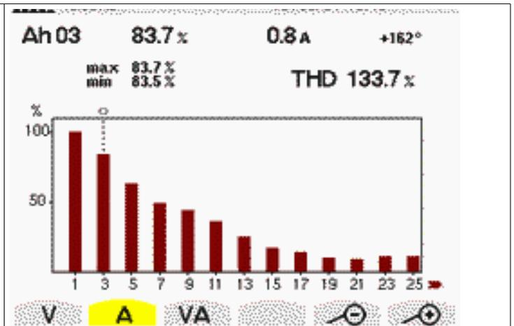
figure 6: spectre du courant de la lampe fluo compacte
