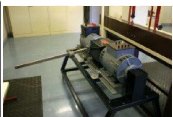
photo 5: banc Mcc/Dynamo balance 3kW
